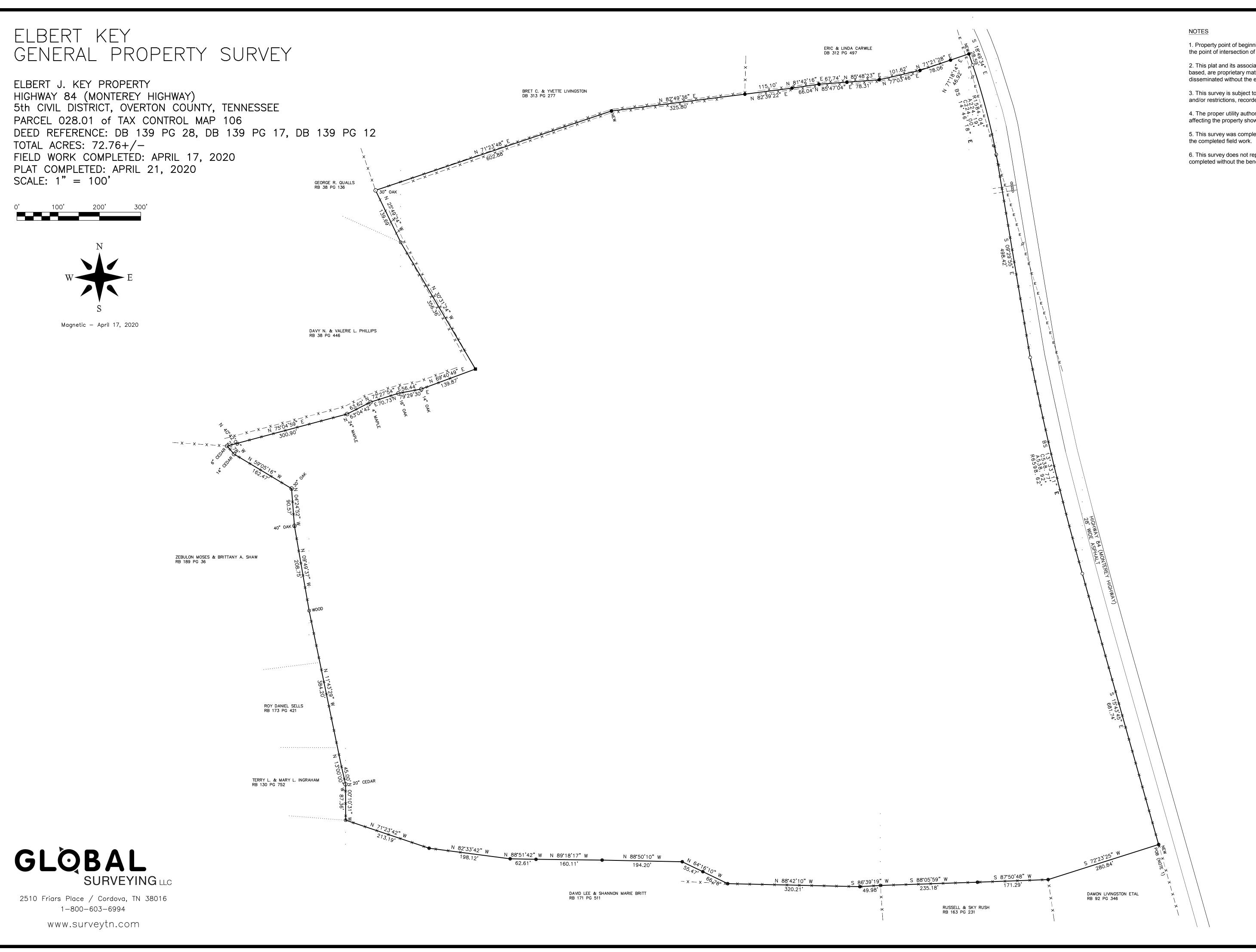
1. Property point of beginning (POB) being N 18°25'44" W a distance of 1108.81' from the point of intersection of the centerlines of State Highway 84 and Dry Hollow Road.
